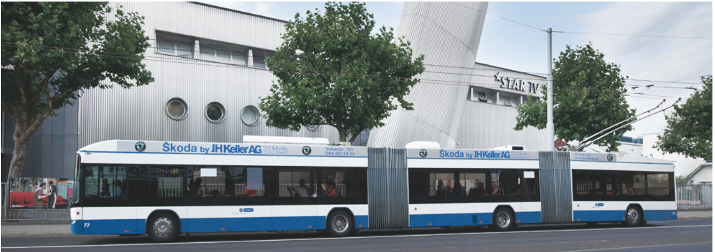
Figure 3: 25-meter-long double-articulated trolleybus (photo by Hess AG)
