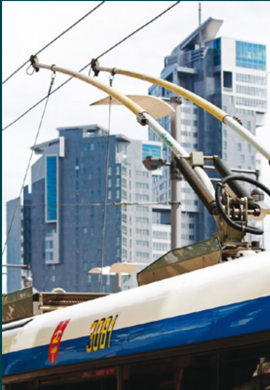
Figure 4: Trolleybus poles (photo by TROLLEY project)
